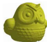
Scanning result of the rubber spray-coated object
