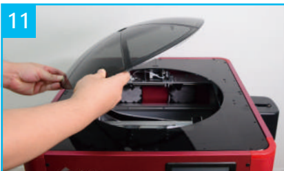
11 Place the top cover down with the guide tube going through the hole in the top.
