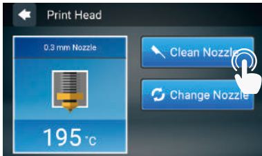
1. Tap Clean Nozzle in the print head section.
