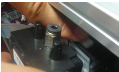
7. Press the white release button to separate the print head.
