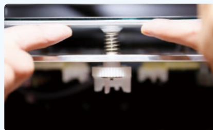
2. Used to 2 thumb to push up the print-bed to release the calibration screw.
