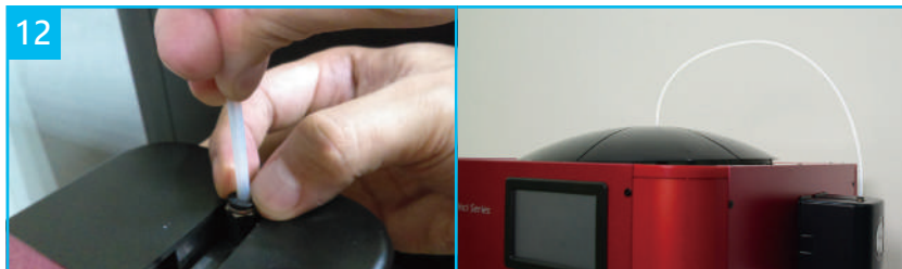
12 Insert the other end of the guide tube into the feed module and secure it tightly.
