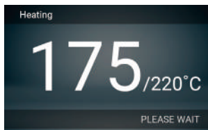
3. The printing operation will start once the print nozzle is warmed up.
