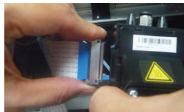
8. Hold the print head with one hand and remove the bus with the other. The removal of the print head is completed.
