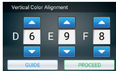
7. For vertical alignment, enter each color's corresponding number. After entering the number, tap PROCEED.
