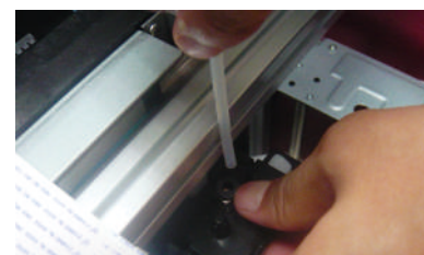
6. Change the print head from above the machine.
