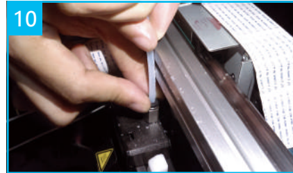
10 Insert the guide tube through the top cover, and then insert one end into the printing module.
