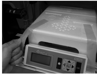
4 Remove the securing styrofoam and fixing tape on the print bed.
