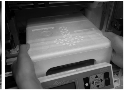
4 Remove the securing styrofoam and fixing tape on the print bed.
